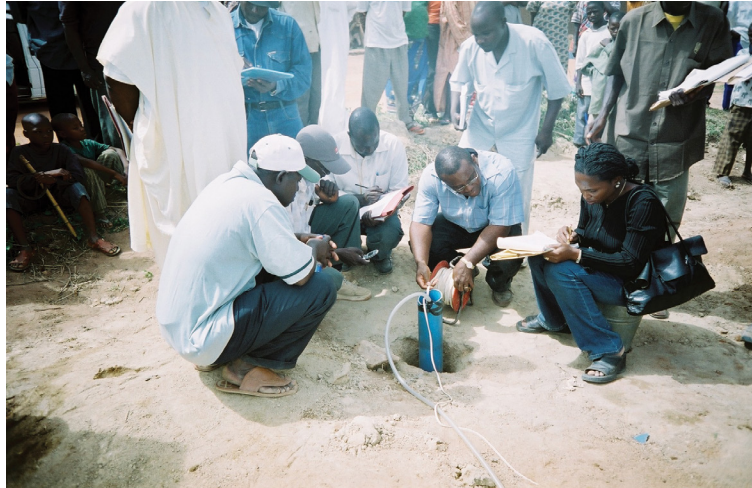
FIGURE 3: Hydrogeologists monitoring a groundwater level in a newly drilled borehole in Nigeria
